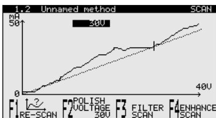
After filtering the current density curve might look like that, and the correct polishing value is easy to define.
