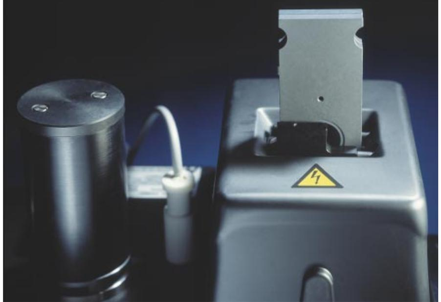
The polishing unit with the electrolyte pump, electronic thermometer and exchangeable specimen holder.
