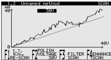
As not all materials display such an easy to analyse current density curve as shown before, both filter and enhance functions are included with the TenuPol-5.
